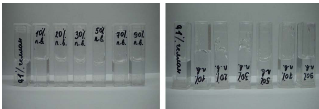
Figure 4. Gelation of 0.1% gellan solution in the presence of 10–90 vol % oilfield saline water at room temperature. [Color figure can be viewed in the online issue, which is available at wileyonlinelibrary.com .]
